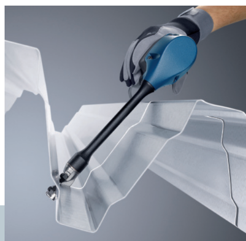
Diagonal cutting on deep corrugated roofing
