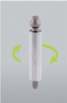
TRUMPF's consumable materials generally have a long service life. In the N 160 models, the wear of the punch is reduced by a rotational movement. This allows for regular wear and tear. The result: surprisingly long service life and low operating costs.
