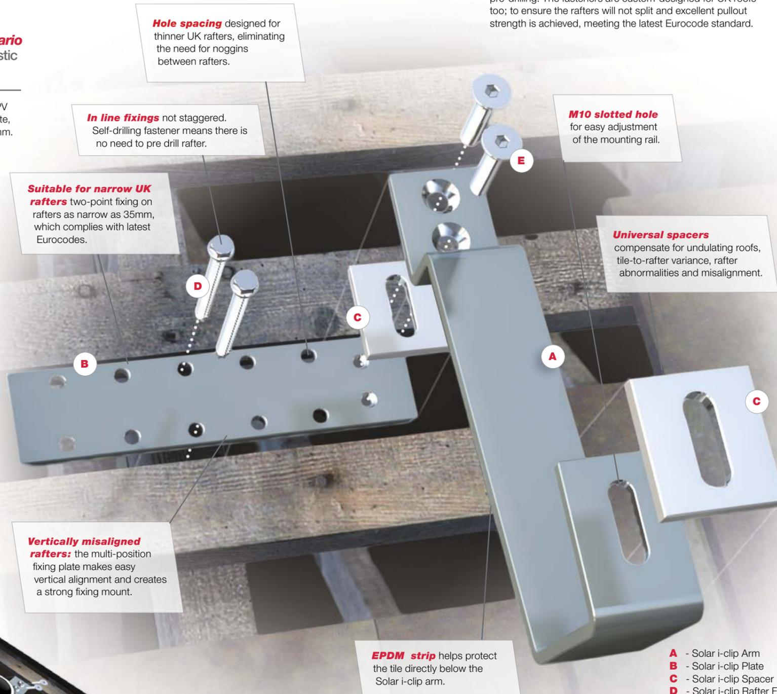
**Vertically misaligned rafters:** the multi-position fixing plate makes easy vertical alignment and creates a strong fixing mount.
