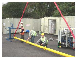
Once the beam is fully assembled in the correct fashion, attach one lifting sling through each of the large top shackles, ensuring that the shackle pin is securely tightened afterwards.
