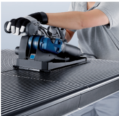
Right-angle cuts using a 90° adjustable blade.
