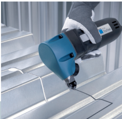
Notching and interior cut-outs
