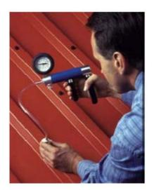
Note washers, which are under driven, may not Provide the desired weather seal. EJOT recommend That all fasteners are vacuum tested after installation To ensure they have been correctly installed.
