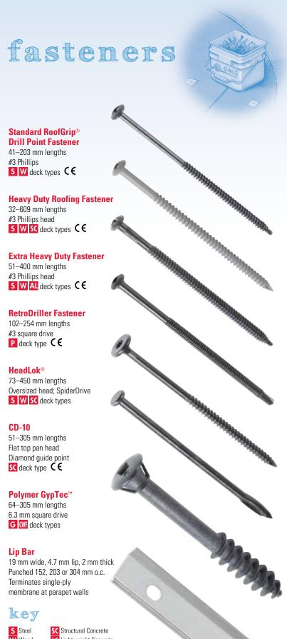
OMG Roofing Products has the industry's widest assortment of specialty roof fixings and plates for virtually every roofing application.
