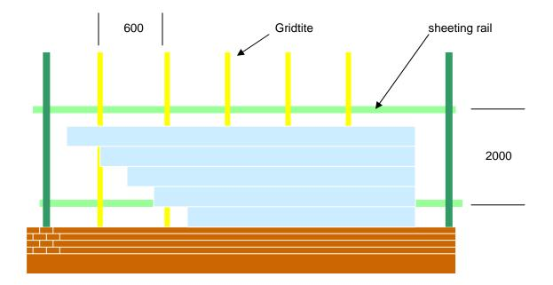
The standard Gridtite <u>bar / bar</u> push fit joint is **not** designed to carry cladding loads applied *along* the bar as is found in upright fixing. Inserting a fastener into the pre-punched holes in the socket joint will lock both bars together and will help to transmit loads.
