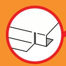
Just cut and turn the tabs under the tile at the base of the Dektite® Aluminium™ for stability. Trim to fit as required.
