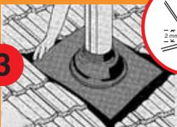
Place upper edge of base under tiles, forming an anti-capillary fold.
