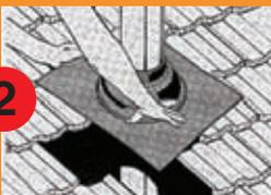
After lubricating the flue with water, slide Dektite® Aluminium™ down to the tile level.
