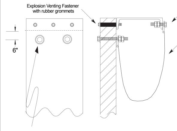
1/2" x 4" stainless steel cable bolt with 2-1/2" OD washer
